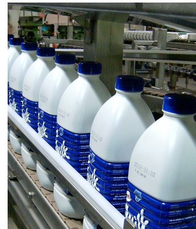
BAT-BUFFER in stainless steel for PET milk bottles.
