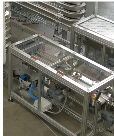
Double BAT-BUFFER for candy boxes. Productivity 200 pcs/min, each.
