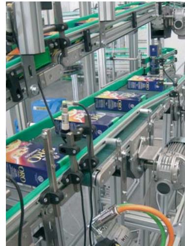
Set of F6 conveyors for phasing and glueing of two rice boxes together
