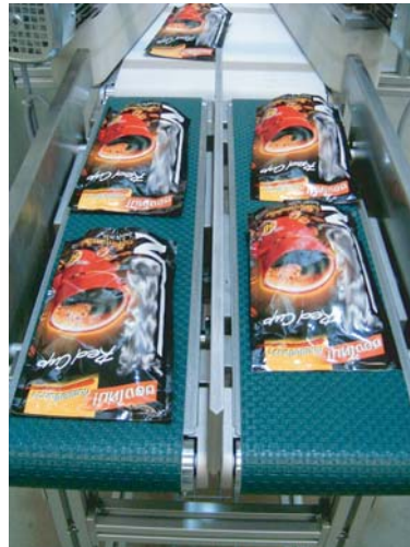
F6 conveyors with high grip belt, for 2 in 1 row unification system of doypacks
