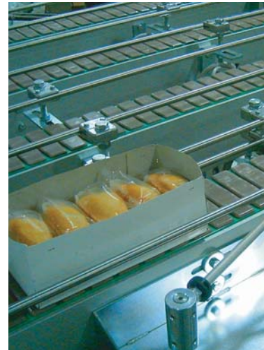
Multiple lines of Jolly-Flex for sweets packaging line
